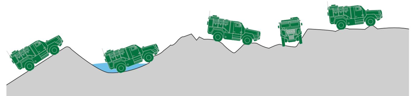
Slope **60 %**      Fording **800 mm**      Trench **900 mm**      Side Slope **30 %**      Step **400 mm**
