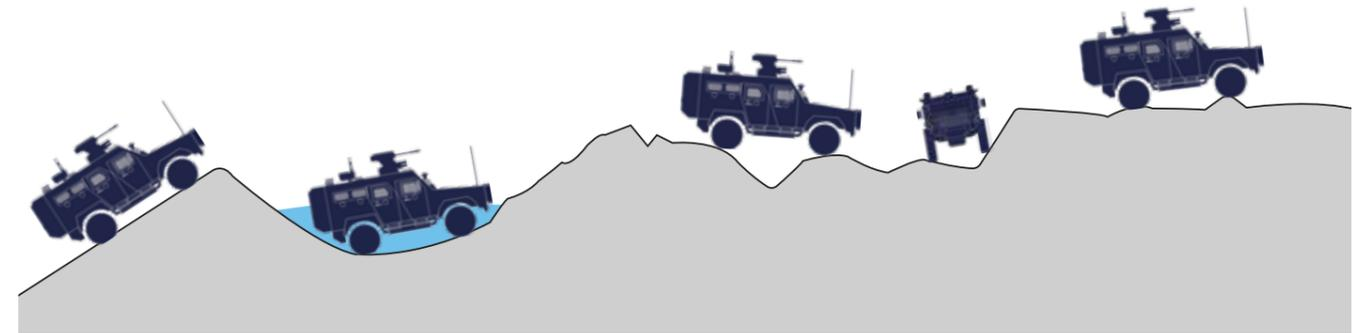
Slope 60 %      Forging 600 mm      Trench 900 mm      Side Slope 30 %      Step 400 mm
