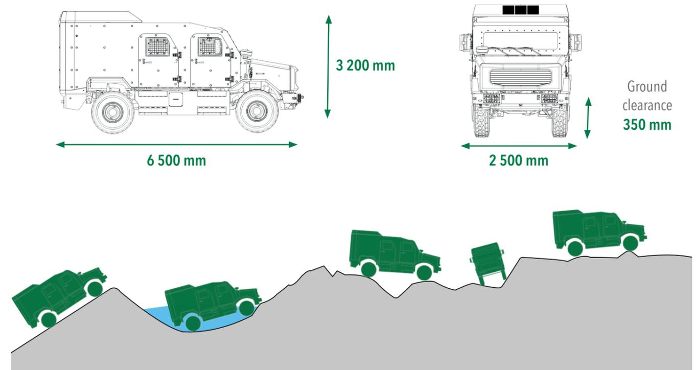
The **ARAM** (Armoured Ambulance) is a **heavily protected mobile** 4x4 ambulance that is **reliable, modular and easily accessible, with extended driving capabilities.**
